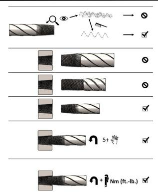
NOTE :Anchors must be assembled with calibrated torque wrench. Torque wrench must be calibrated at least every 24 months (+/- 15%). Thread does not need to be flush with end of anchor. Thread may be +/- 2 threads from backside of anchor
